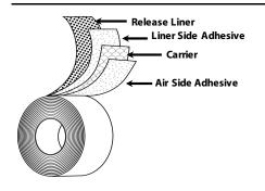
Liner:74# Polycoated KraftLiner Side Adhesive:Rubber (1917)Backing/Carrier:0.5 mil PET FilmAir Side Adhesive:Rubber (1917)
