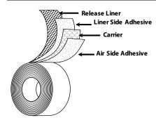
Liner:12pt Polycoated KraftLiner Side Adhesive:Rubber (I920)Backing/Carrier:0.5 mil PET FilmAir Side Adhesive:Acrylic (I639)Specifications:Chrysler PF-10770(NC); Toyota TSK6712G<br/>GM 3607M Type1, 3622M Type IV<br/>Ford ESA-M11P19-A, ESB-M3G76-B2, ESH-<br/>M11P19-B<br/>Delphi SD2-324 4.1.1, 4.1.4,4.3.3
