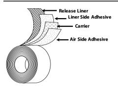
Liner:12pt Poly-coated KraftLiner Side Adhesive:Rubber (I915)Backing/Carrier:0.5 mil PET FilmAir Side Adhesive:Acrylic (I623)Specifications:Chrysler PF-10770(NC); GM3622M Type<br/>IV, Cycle E; GM3607M Type I, Ford ESA-<br/>M11P19-A, ESB-M3G76-B2, ESB-M11P8-A,<br/>ESH-M11P19-B, WSF-M11P8-A2; Delphi SD2-
