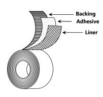
Backing:1/16" white, crosslinked polyethylene foamAdhesive:Non-Sensitizing Acrylic (M108)Liner:74lb bleached polycoated kraft, silicone<br/>treated on one side
