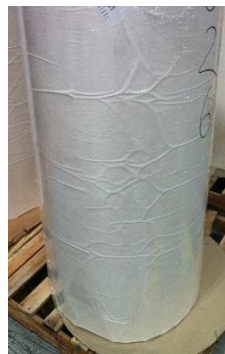
Rolls of tape showing the cockling phenomenon
