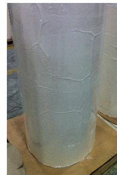
Rolls of tape showing the cockling phenomenon
